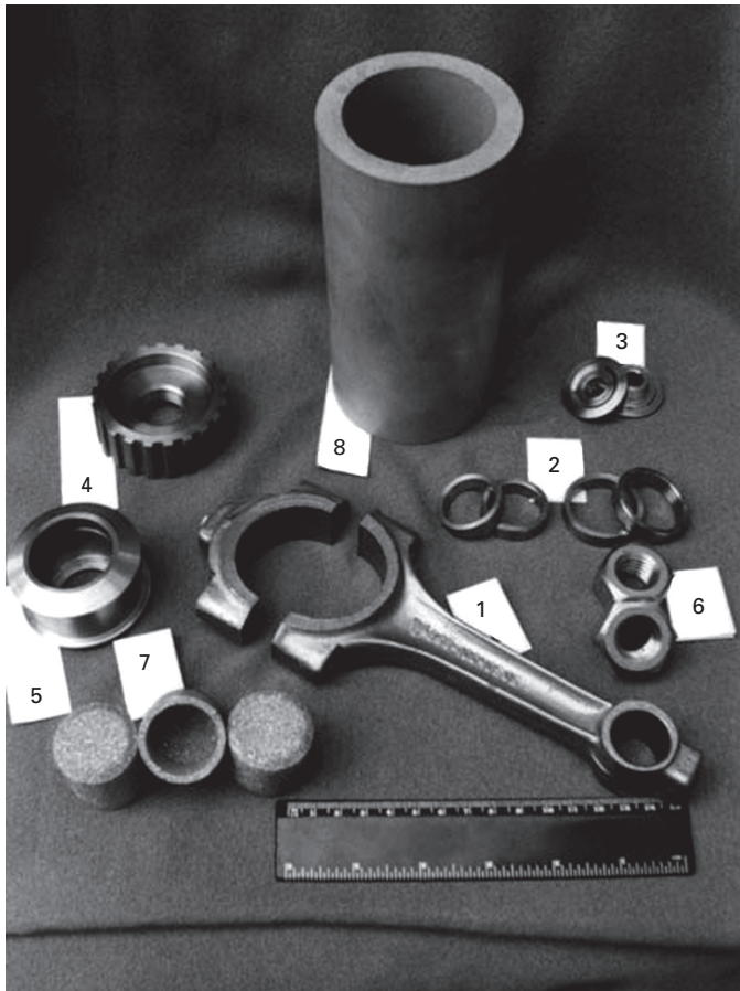
8.13 Ti-6Al-4V parts produced using a press-and-sinter approach and titanium hydride: (1) connecting rod with big end cap, (2) saddles of inlet and exhaust valves, (3) plate of valve spring, (4) driving pulley of distributing shaft, (5) roller of strap tension gear, (6) screw nut, (7) embedding filter, fuel pump, and (8) embedding filter (courtesy Ukrainian Academy of Sciences).
