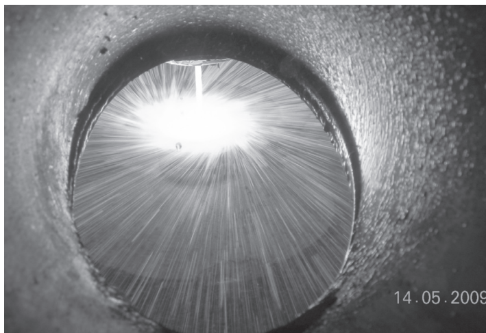
1.10 Centrifugal atomisation of steel at 70 \text{ kg min}^{-1} to \sim 100 \text{ }\mu\text{m} powder.
