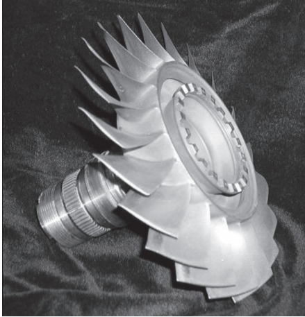
8.35 ALM repair of gas turbine components.
