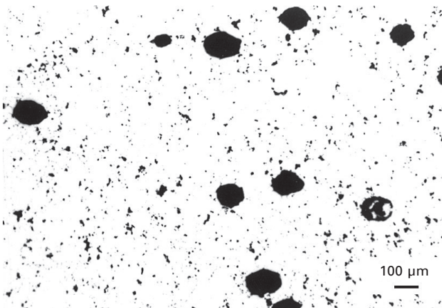
7.8 Secondary pores in sintered Fe-3% Cu.
