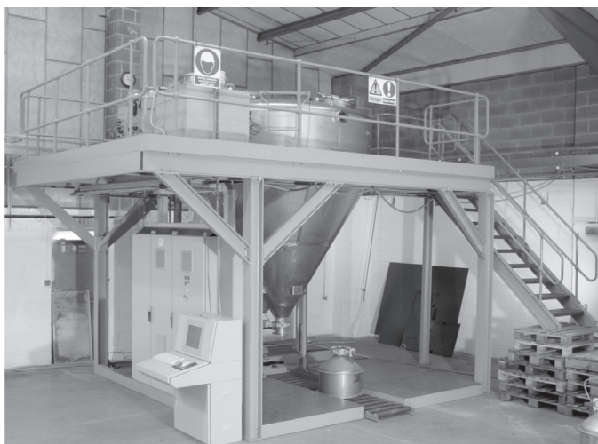
1.7 Industrial centrifugal atomisation system for electronic solder powders.
