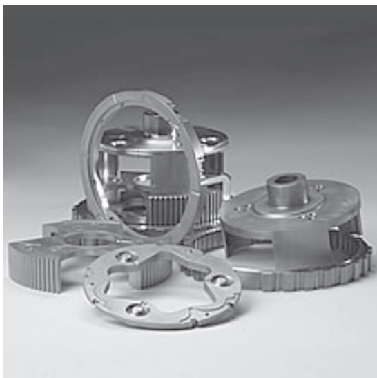
17.29 Carrier and one-way rocker clutch assembly for automatic transmission (credit MPIF).
