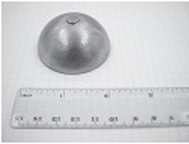
12.7 Pure W dome part sintered in microwave at 1800°C for 30 mins in pure hydrogen.
