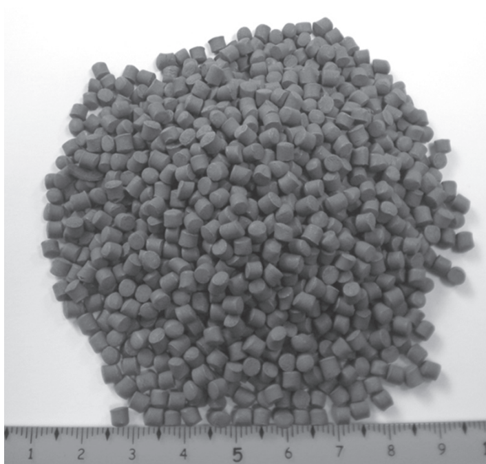
6.9 Ti64 commercial feedstock pellets that are ready for metal injection. The feedstock is available under the product name polyMIM®.
