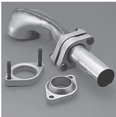
17.15 Manifold flange and exhaust converter outlet flange.
