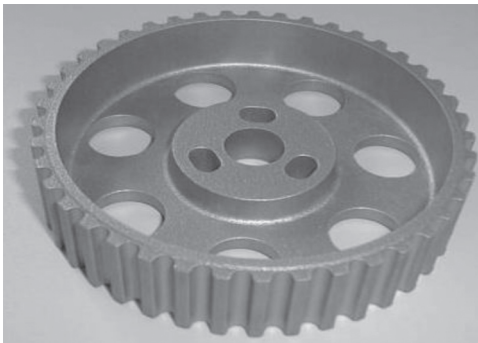
8.32 Automotive pulley prototype fabricated by ALM.
